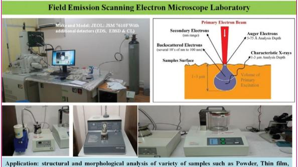
Application: structural and morphological analysis of variety of samples such as Powder, Thin film, Powder pallet, Biological, Geological, Fossils, Nanomaterials, Polymers, Ceramics, Metals, Dental materials, Pharmaceuticals etc
